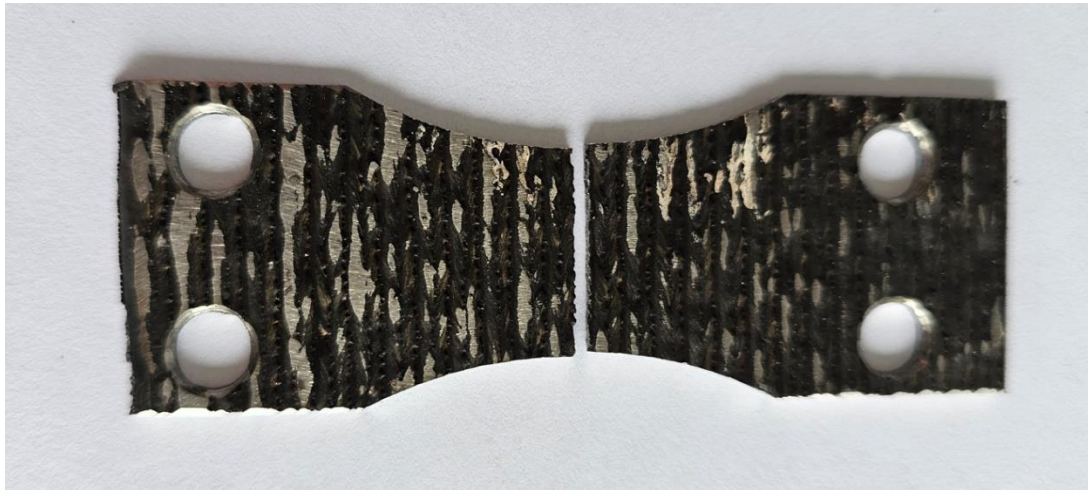
Fig. 6. As-built specimen fractured in fatigue test.
