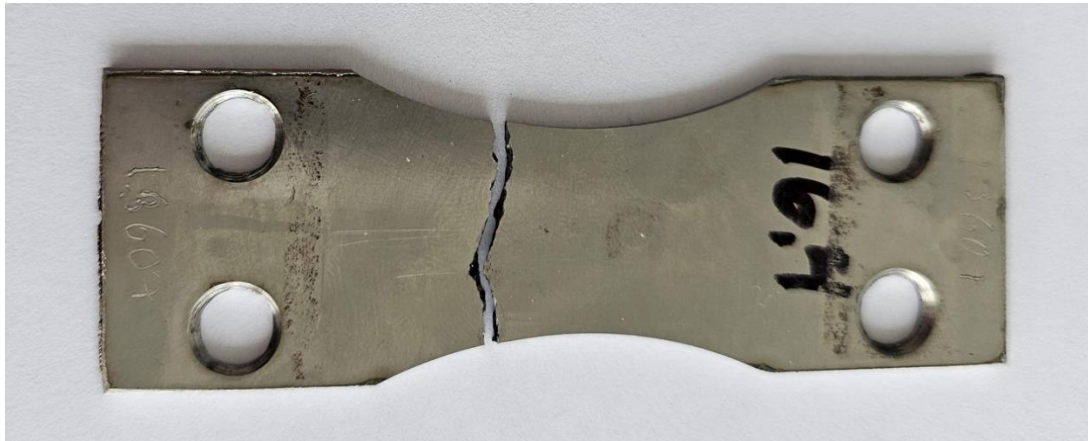
Fig. 5. The machined specimen fractured in fatigue test.
