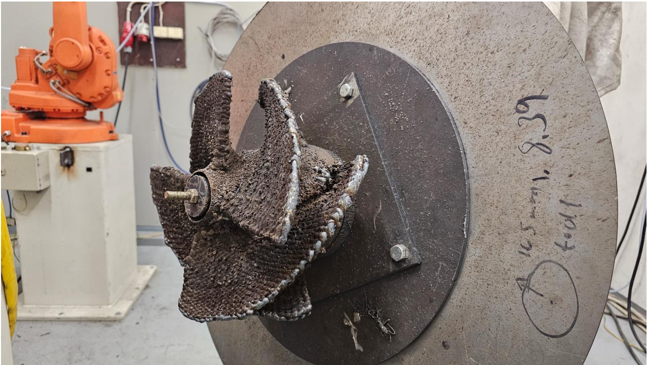
Fig. 2. WAAM fabricated complex geometry.
