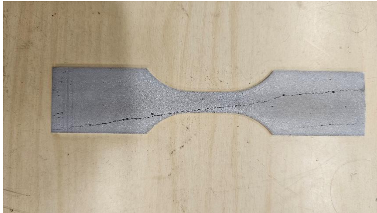
Fig. 3. Discarded fatigue sample.
